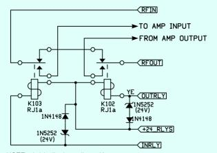
NOTE: Add diodes directly across the vacuum relay coils. Be careful to observe correct orientation. (The cathodes are the banded ends of the diodes.)
